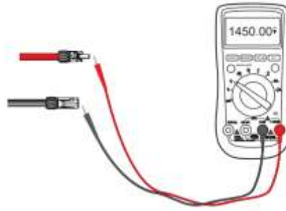
Figure 4-14 Ensure the polarities of the DC cables
